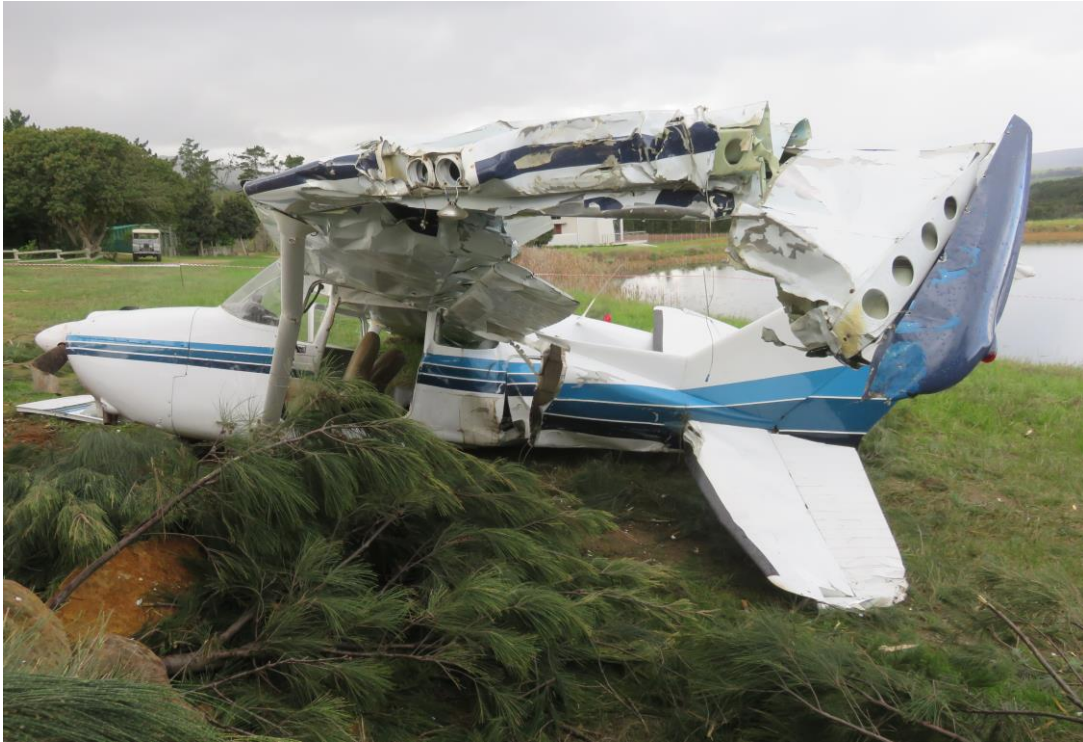
Figure 14: The left-wing was severely deformed during the impact sequence.
