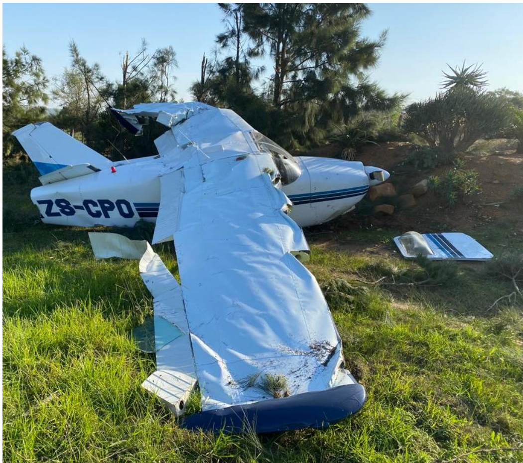
Figure 11: Damage on the leading edge of the right wing following impact with the trees.
