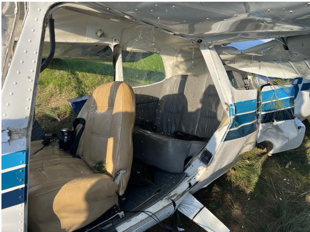
Figure 13: Fuel leaking from the ruptured left-wing tank. (Source: Passenger)
