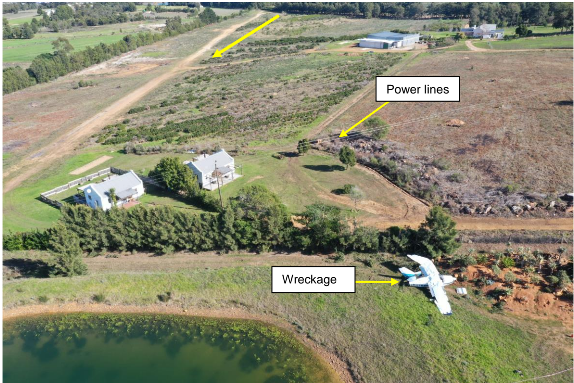
Figure 10: The runway, power lines and wreckage. (Source: AAS drone footage)
